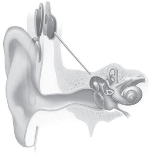
Schematic diagram of a cochlear implant. The external components consist of a microphone, a sound processor, and a transmitter of power and processed signals. The internal components consist of a receiver and stimulator, along with an array of electrodes that can be seen wound up within the cochlea in the figure. (Image: Creative Commons).
